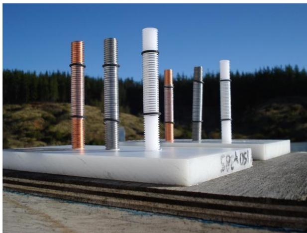
**Figure 1.** Wire-on-bolt assembly.
